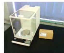
Weighing scale used and verification weights
